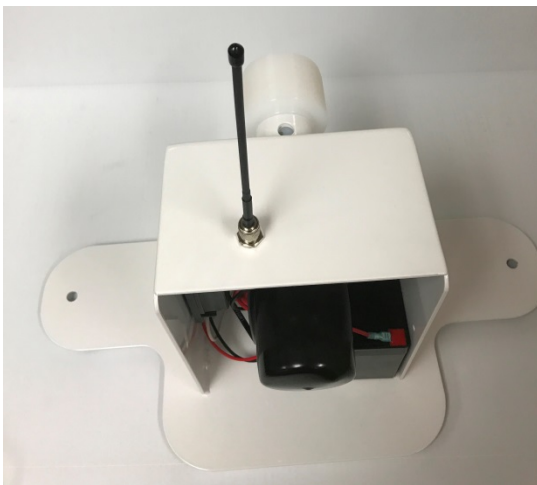
Photo of Drive side stand with Antenna Installed
